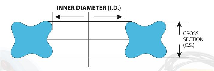
X RINGS ALSO KNOWN AS FOUR LOBED RINGS ARE USED IN VARIETY OF DYNAMIC AND STATIC SEALING APPLICATIONS
